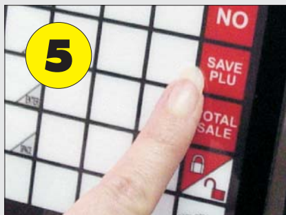
Press "SAVE PLU" key, then assign the product on the memory-key you want to set the product, you can chose any of the 72 direct access.
